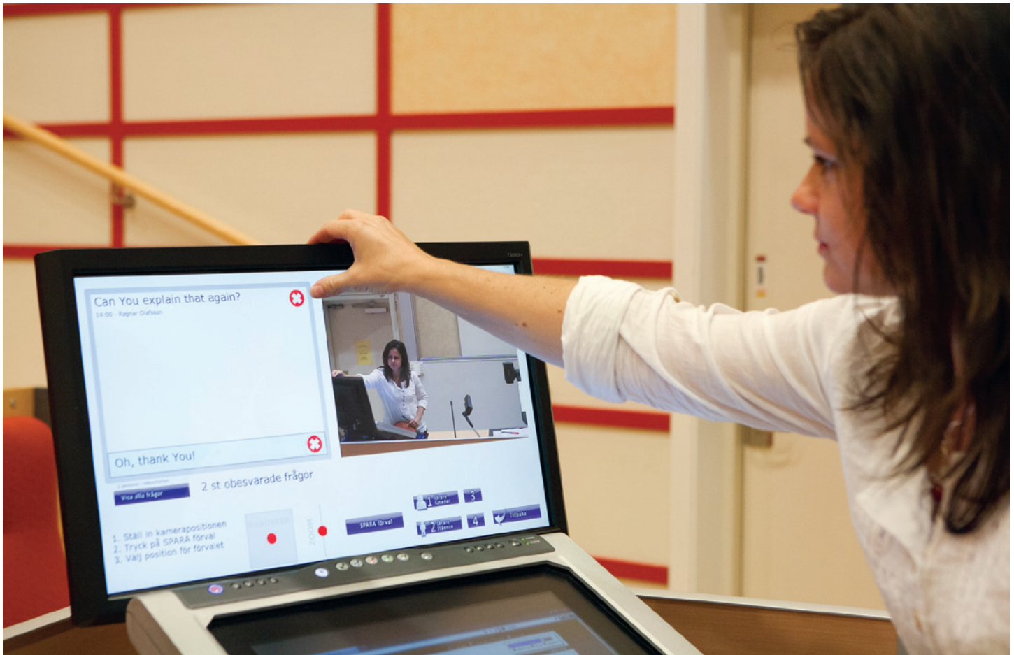
A touchpanel provides control over classroom media, manages questions submitted using chat, and presents a live view of streamed content.
