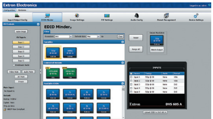
All models of the DVS 605 include built-in Web pages that enable easy setup and remote access for Help Desk assistance.
