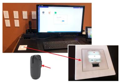
RCP 101 Remote Control Panel for SMP 351 Streaming Media Processor is located on the AV operator desk, providing a convenient location to insert a USB memory stick and to start, stop, pause, lecture capture and streaming. Presenters can also control start, stop, and pause from a button on their VoiceLift Pro pendant mic.
