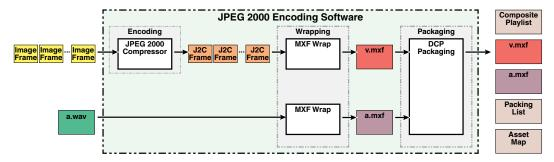
Figure 19. Encoding, Wrapping, and Packaging Process
