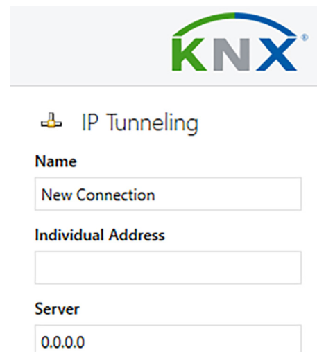
Figure 5. Changing Device Address in ETS
