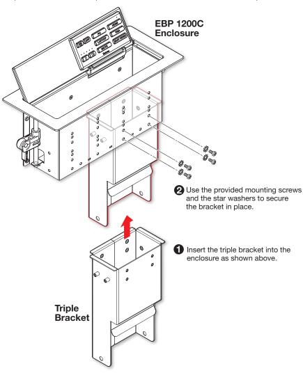
**NOTE:** Optionally, the Triple Bracket can be turned 180 degrees and mounted, depending on the application need.
