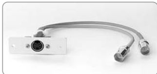
IN9485B / IN9485W Single space AV connector module (black / white): 4-pin mini DIN female on front and (2) female BNC with 6" pigtails on back
