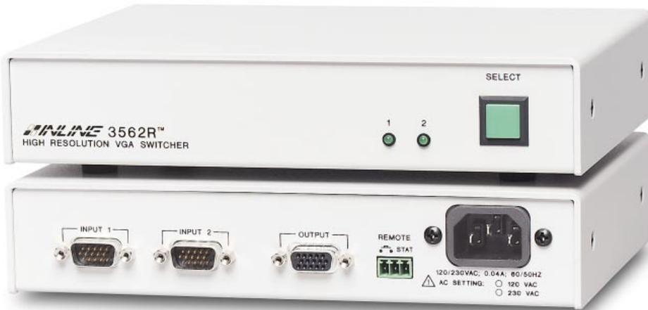
The **IN3562R** is an ultra-high resolution VGA switcher designed to select between two computers with VGA / SVGA / XGA graphics cards, routing the selected input to a data display such as a data monitor, presentation monitor, or data projector. The **IN3562R** features 15-Pin HD connectors for inputs and output and connects directly to VGA-type video sources and displays using high resolution coaxial VGA extension cables such as the **IN8000** Series.
